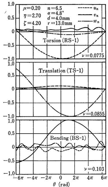
Fig. 7 The change of vibration modes with mass ratio-(1)
