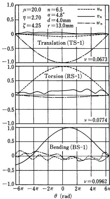
Fig. 9 The change of vibration modes with mass ratio-(3)
