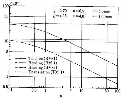
Fig. 5 Dimensionless natural frequency vs. mass ratio-(1)
