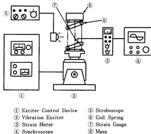
Fig. 10 Diagram of measuring system for experiment
