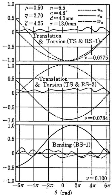
Fig. 8 The change of vibration modes with mass ratio-(2)
