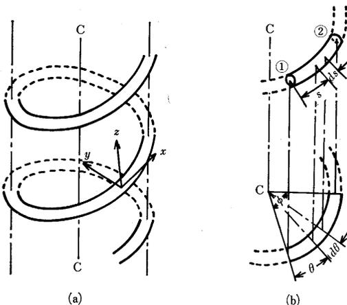
Fig. 1 Co-ordinate (a) and spring element (b)
