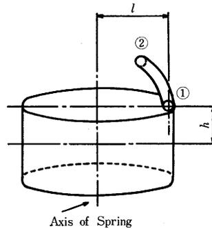
Fig. 2 Rigid body-spring element
