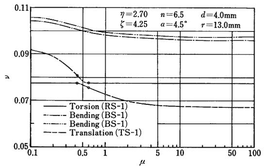
Fig. 6 Dimensionless natural frequency vs. mass ratio-(2)
