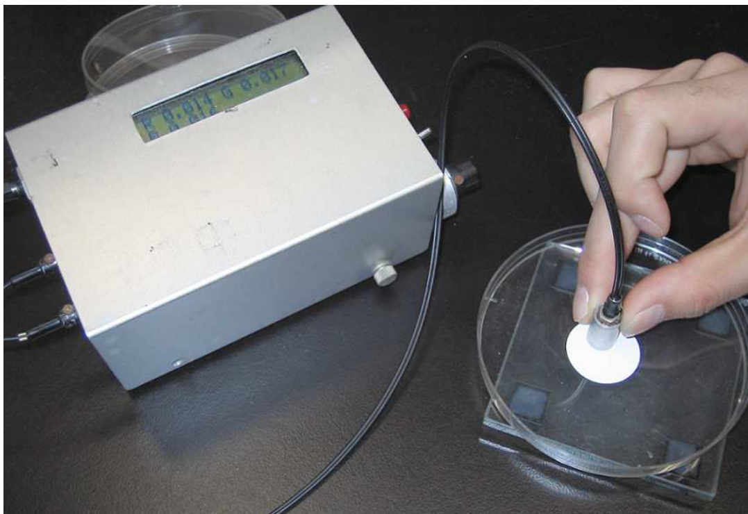
Fig. 2.2 Measurement of reflection-absorption by portable colorimeter.
