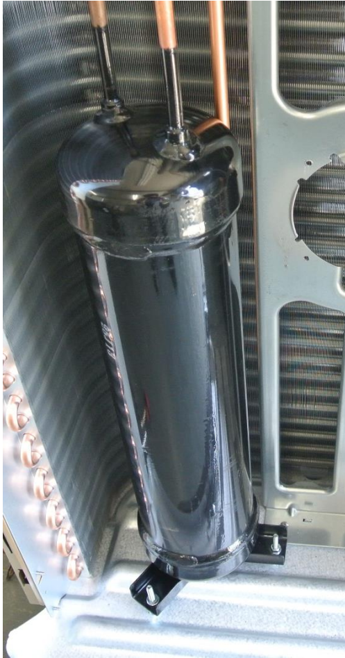
Figure 2.12 Picture of receiver tank
