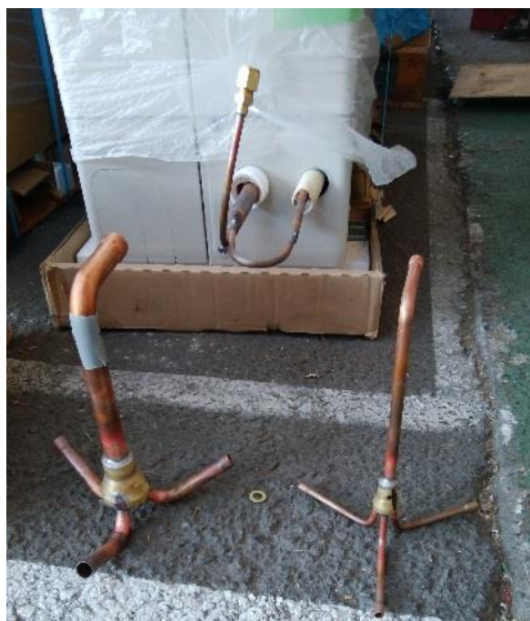
Figure 3.39 Picture of distributor
