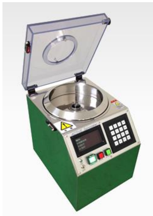
Fig. 3-2. A picture of spin coater used in the experiment ( http://www.acti-ve.co.jp/spincoater/standard/act220d2.html )
