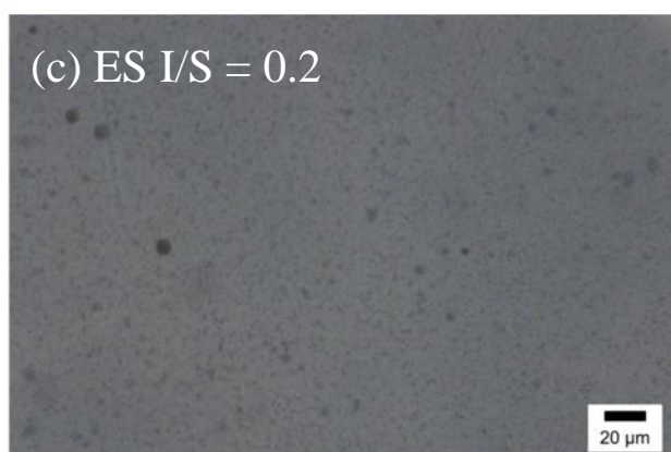
Fig. 4-1 Photographic images of droplets on the membrane prepared (a) by the PSS method with the I/S = 0.7 ink, (b) by the ES method with the I/S = 0.7 ink and (c) by the ES method with the I/S = 0.2 ink.
