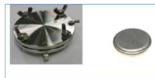
Fig. 4-11 Coin cell preparation
