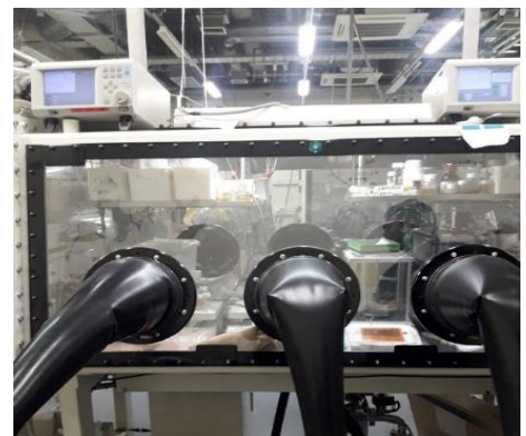
Fig. 4-5 Argon filled globe box used for coin-cell preparation.
