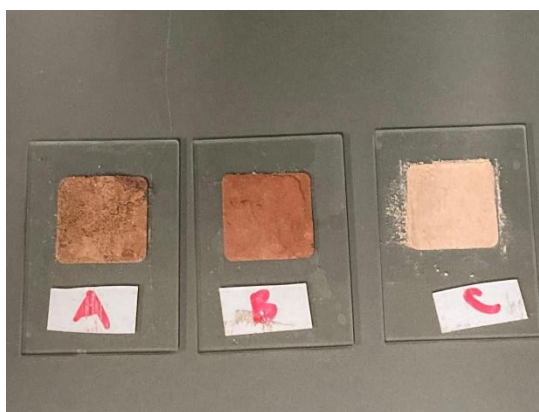
Photo 3.7 Oriented powder in sample holder
