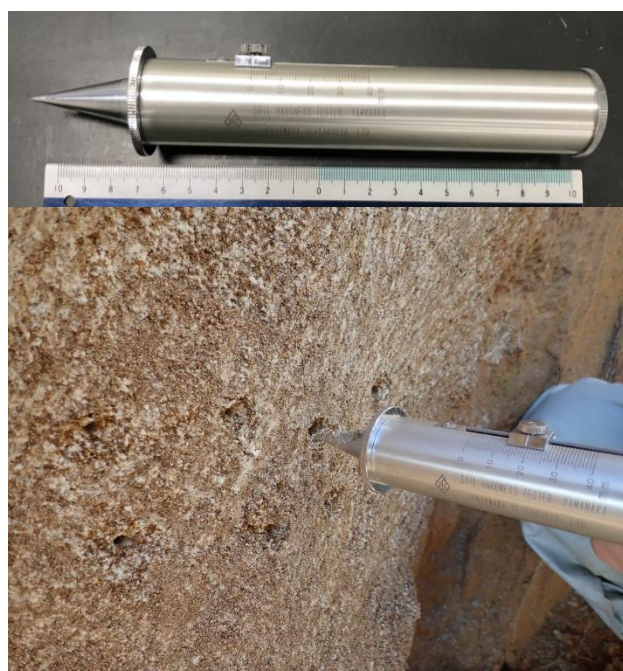
Photo 3.2 Measuring soil hardness using a Yamanaka-type soil hardness meter
