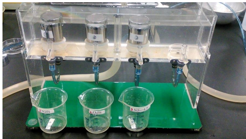
Photo 3.6 Saturated hydraulic conductivity test (Constant water level test)
