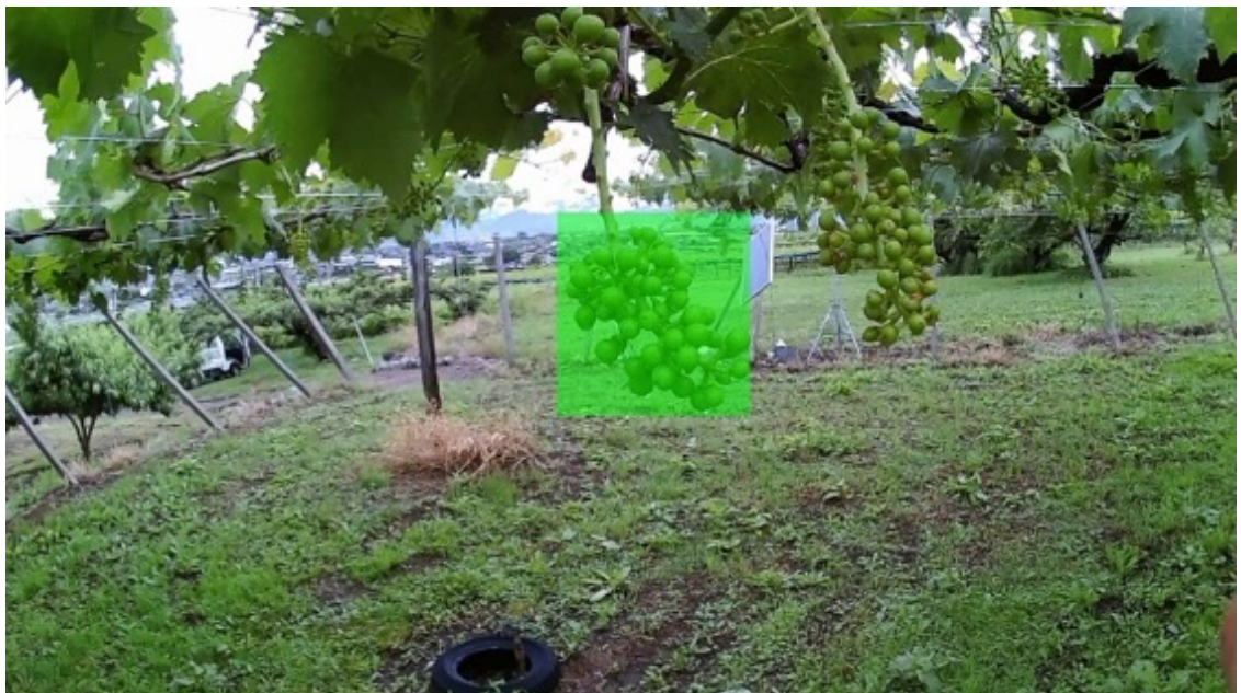
Figure 4.9 An example in which only the working bunch is detected by applying the proposed location-sensitive HTC and post-processing.
