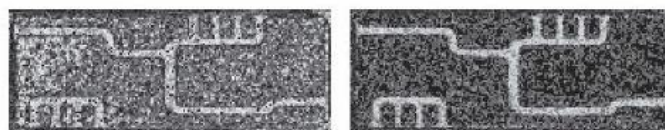
(a) Before heat cycle test. (b) After 6,400 cycle.
